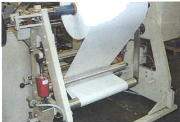
Auto tension control & web alignment
