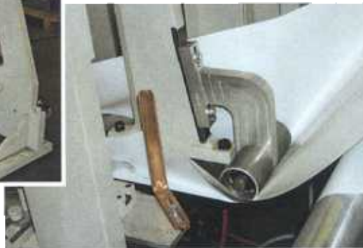
Reduced friction "live heel" former
