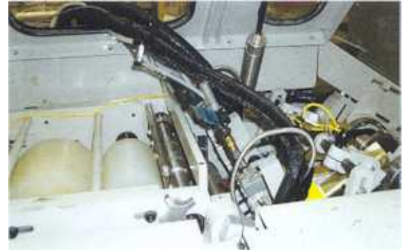
Enclosed hot melt seam seal and bottom paste systems
